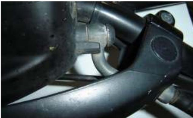
Above is front master cylinder banjo connection. At right is the 'T' piece to split hoses to each of the front calipers. We chucked all the brake lines and fitted a new braided set from HEL Performance that are all one piece. About \$320AUD incl tax.
