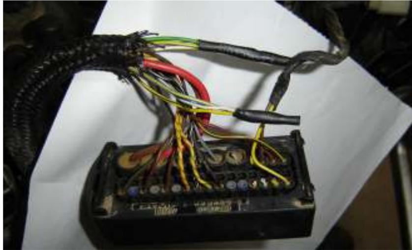
This shows the servo unit plug with the wires snipped off and rejoined as per the rewiring diagram. They were soldered and triple heat shrink wrapped.
