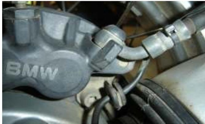
Above left shows the existing rear hose. It can be transferred direct to the master cylinder where the steel line is connected. Above is the rear caliper banjo. Below left is one of the front caliper banjos. Below is brake line connection under the tank on the right side of the steering head. If you aren't fitting new one piece lines you need to replace this with a non ABS fitting.
